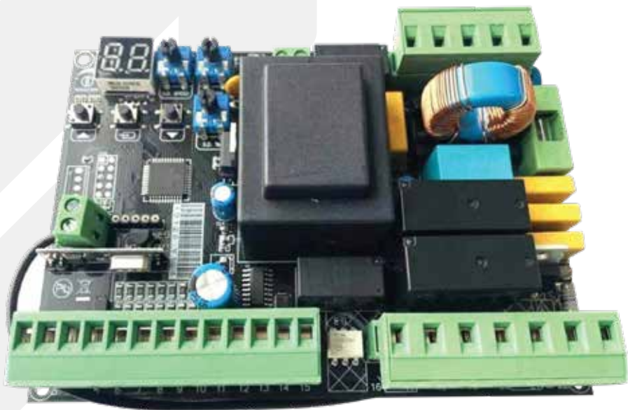
Control unit for sliding gate motor and automatic barrier designed to satisfy needs and expectations in terms of performance and functionalities in the automation of automatic barriers and sliding gates.
